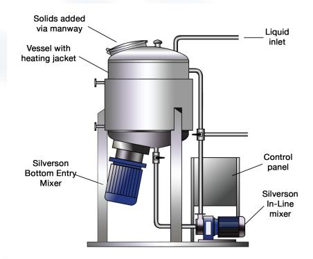
In a typical operating procedure the vessel is first charged with the base fluid, most commonly water. This is heated to the required working temperature before the Bottom Entry mixer is started and the product for reclaim is added. Large solids can be added without the need for pre-grinding. The mixer exerts a powerful suction which draws the materials down into the workhead, where they are rapidly reduced to granular size.
