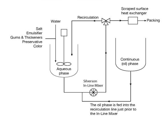
The aqueous phase ingredients are added to the vessel and recirculated through the self-pumping In-Line mixer which disperses and hydrates the materials, rapidly producing a homogeneous agglomerate-free mix.
