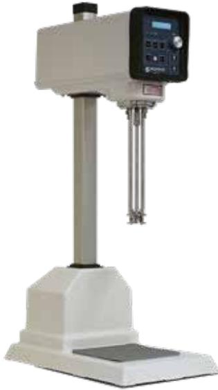
Silverson Laboratory mixers are suitable for the widest range of applications - mixing, emulsifying, homogenizing, disintegrating, and dissolving. With a capacity from 1ml up to 12 liters and the ability to mix in-line with flow rates of up to 20 liters/minute, they offer excellent reproducibility when scaling up and provide an accurate means of forecasting the performance of larger Silverson machines under full-scale working conditions.
